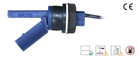
**How it works** Movement of the magnetic float opens/closes a hermetically sealed contact (reed switch).
